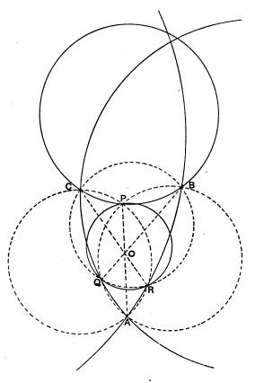
Thus let us consider three circles BCQR, CARP, ABPQ, intersecting in the three pairs of points A, P; B, Q; C, R; each pair being inverse points with respect to the circle which cuts the three circles orthogonally. It follows that the circle PQR is the Hart circle of the triangle ABC formed by the circular arcs BPC, CQA, ARB.
